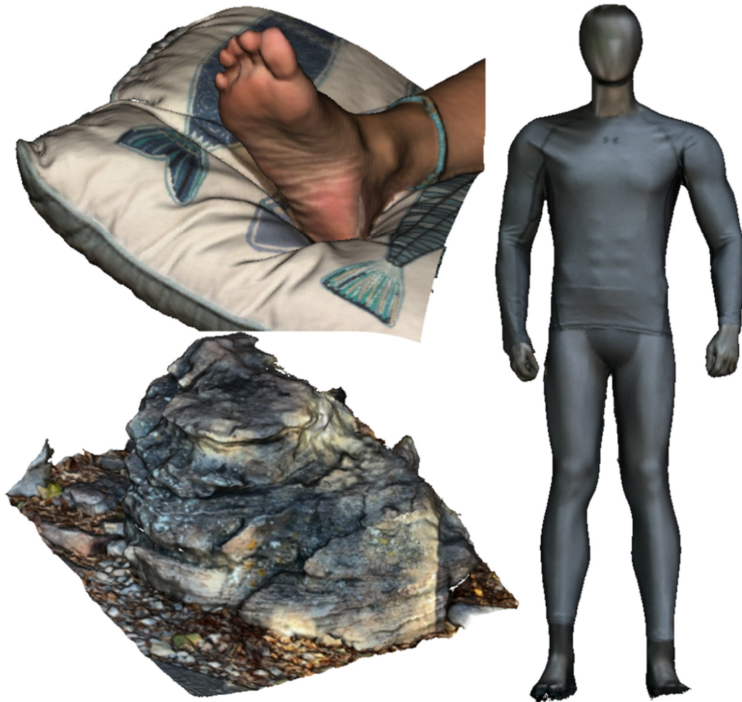
Figure 1: Sample scans performed using the Structure Sensor 3. Top left: female right foot, size 7.5 (US). Bottom left: Large rock (1.4m wide), captured outdoors during daylight. Right: full-body scan of a large mannequin (1.94m tall).
