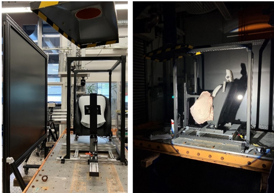
Figure 5 modified replica of the test bench for the side airbag
